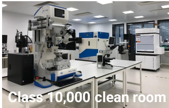
Tressky T-3002-PRO Die bonder Pressure and pressure less sintering process
