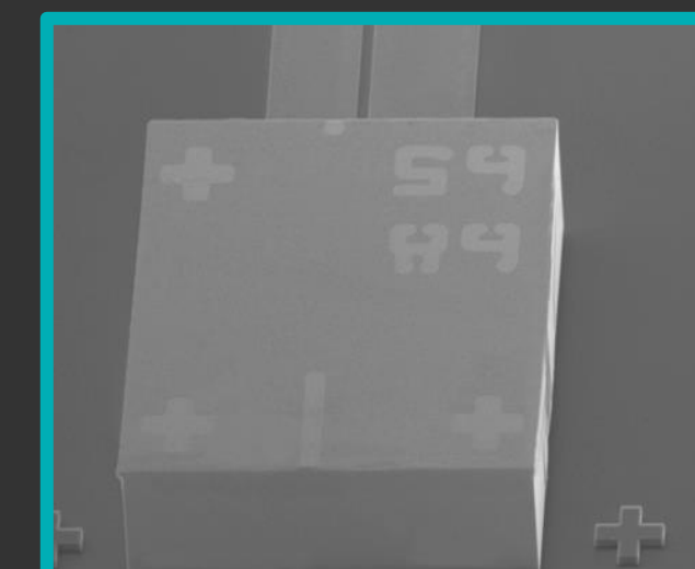
Back-side alignment fiducials and chip IDs
