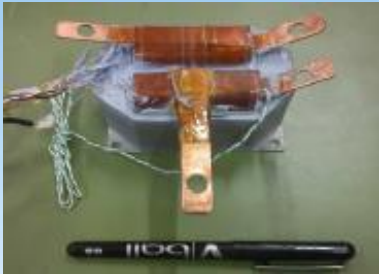
Potted inductor with embedded thermal sensors
