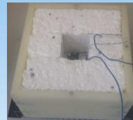
Test rig measures sample's thermal conductivity
