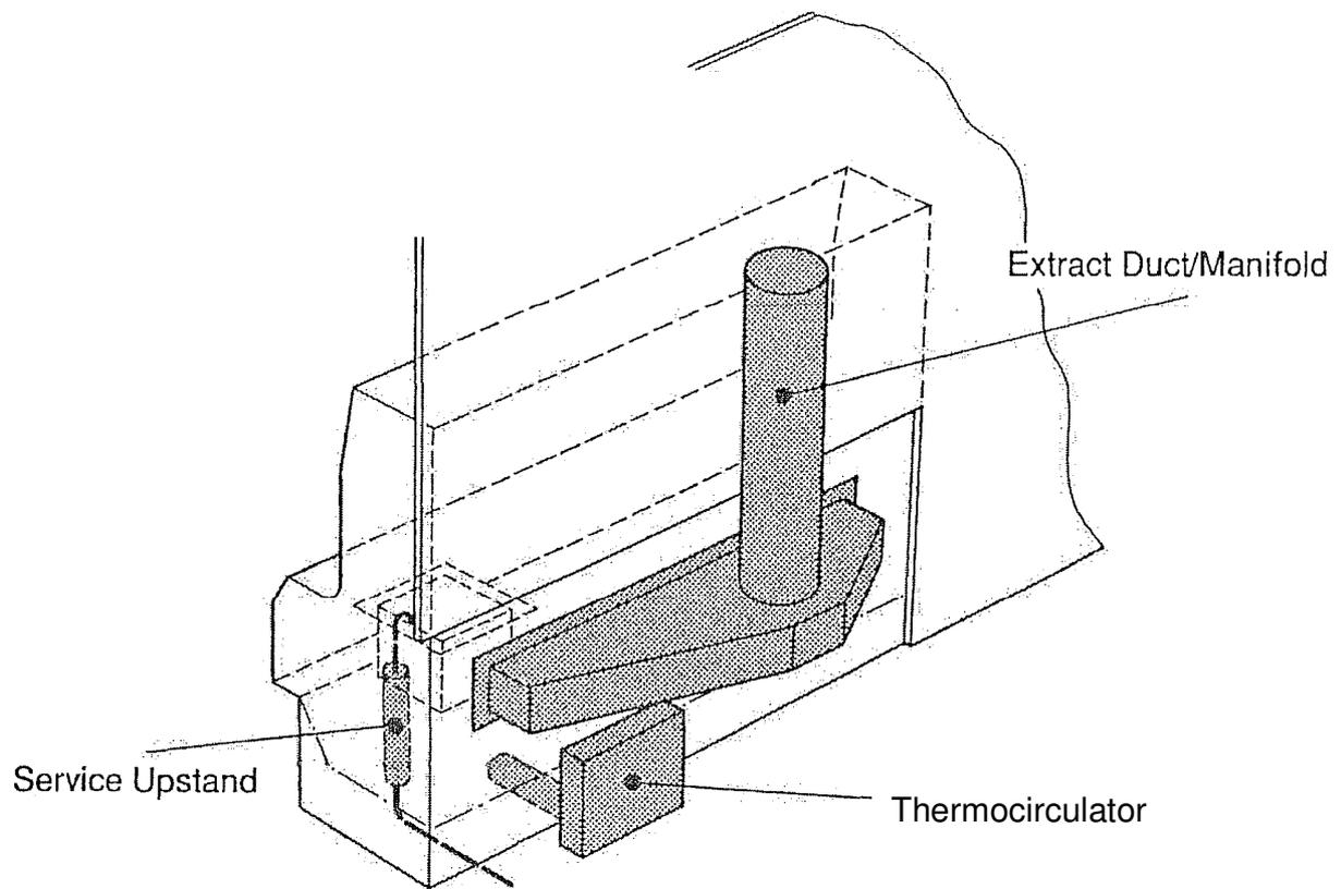
APPENDIX A: 3      CHEMICAL WORKSTATION WITH VERTICAL LAMINAR FLOW
